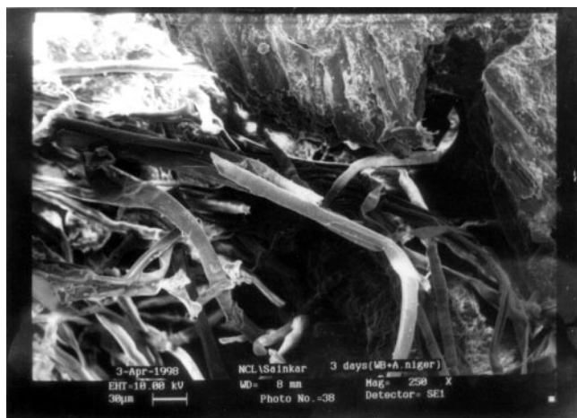
Figure 6 Scanning electron micrograph of wheat bran degradation by Aspergillus niger during SSF after 3 days of fermentation. Marker, magnification ( \times 250 ).
